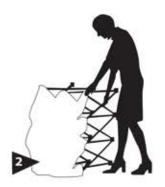
Ensure "adjustable feet" of frame are on the floor. Pull up display into upright position.
